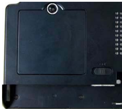
Fig. 4 Removing the cover of the mini PCI card
